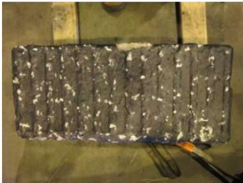
Figure 2.2 Section of concrete tie showing chipped off black paint in areas of ballast particle contact. (FRA Task Order 225)
