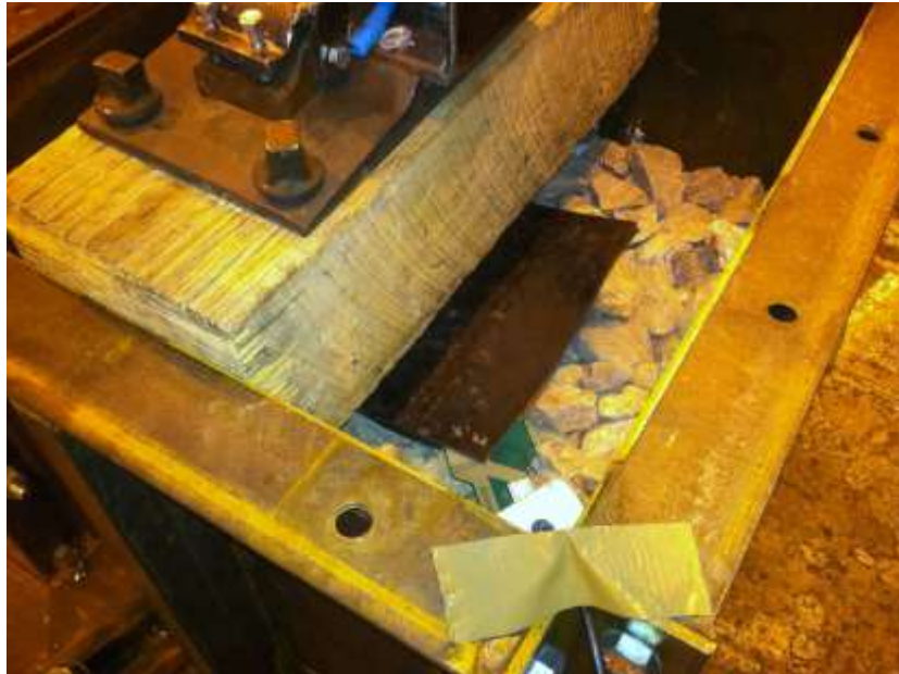
Figure 5.5 Detail of MBTSS sensor/protection location
